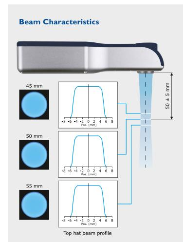
To guarantee the high level of safety the beam of the PXL SAPPHIRE 318 has a wasteline at a distance of 50 mm from the optics and a depth of focus of approx. +/- 5 mm.
