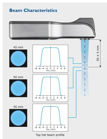
To guarantee the high level of safety the beam of the PXL PLATINUM 330 has a wasteline at a distance of 50 mm from the optics and a depth of focus of approx. +/- 5 mm.
